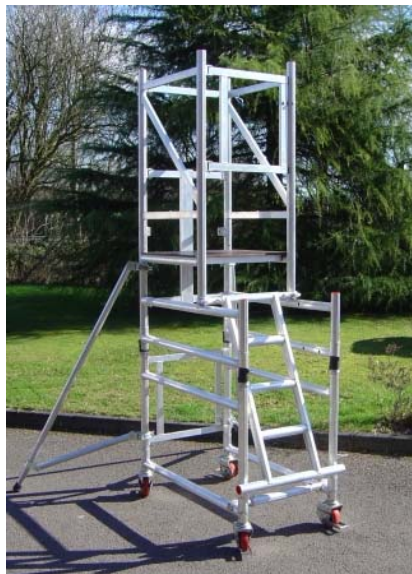
Height Booster Kit raises all platform and working heights by 0.75m. Folding base frame fits underneath the standard SiteMate900. Kit includes Booster frame, access ladder and two stabilisers.
