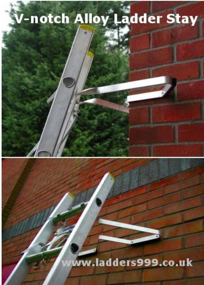
**V-Notch Stay (WSTAYV)** ... large V-notch allows it to span around downpipes or rest on corners of buildings - a big advantage over the old flat front models. Keeps top of ladder 300mm / 12" off the wall and away from fragile plastic gutters. Also useful when working under eaves. Overall width 640mm / 25" with rubber pads on face of stay prevent damage to building. Attachment is rapid and secure with a large spring hook. No tools required.
