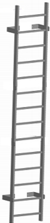
Fixed ladders above 3.0m should have hoops or arrestor device
