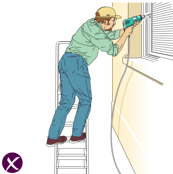
Figure 3b Incorrect - rungs side-on to work activity
