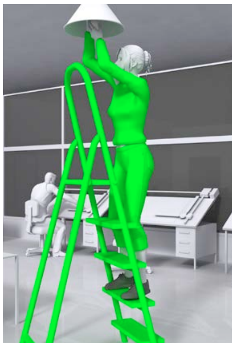
Figure 5 Example where two hands need to be free for a brief period for light work. Keep two feet on the same step and the body (knees or chest) supported by the stepladder to maintain three points of contact. Make sure a safe handhold is available
