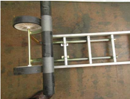
Ridge Hook can be fitted at top end to prevent movement but is only necessary on very steep pitches
