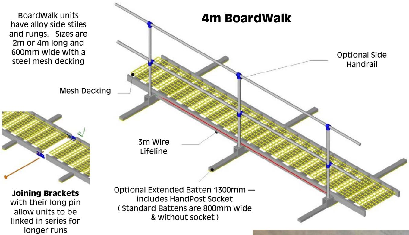
**Joining Brackets** with their long pin allow units to be linked in series for longer runs
