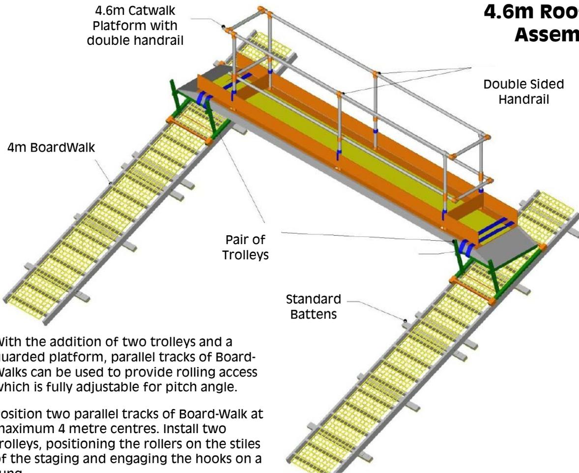
With the addition of two trolleys and a guarded platform, parallel tracks of Board-Walks can be used to provide rolling access which is fully adjustable for pitch angle.
