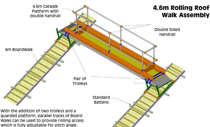
Position two parallel tracks of Board-Walk at maximum 4 metre centres. Install two trolleys, positioning the rollers on the stiles of the staging and engaging the hooks on a
