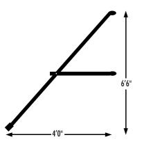
Saturn Tower outriggers are fitted with scaffold type couplers and wing-nuts (spanner not required).
