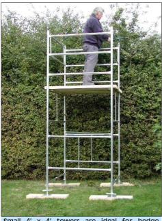
Small 4' x 4' towers are ideal for hedge trimming, here with adjustable legs for levelling. This 6ft platform height tower provides a safe, stable platform for reaching up to 12ft high. Much safer than stepladders!
