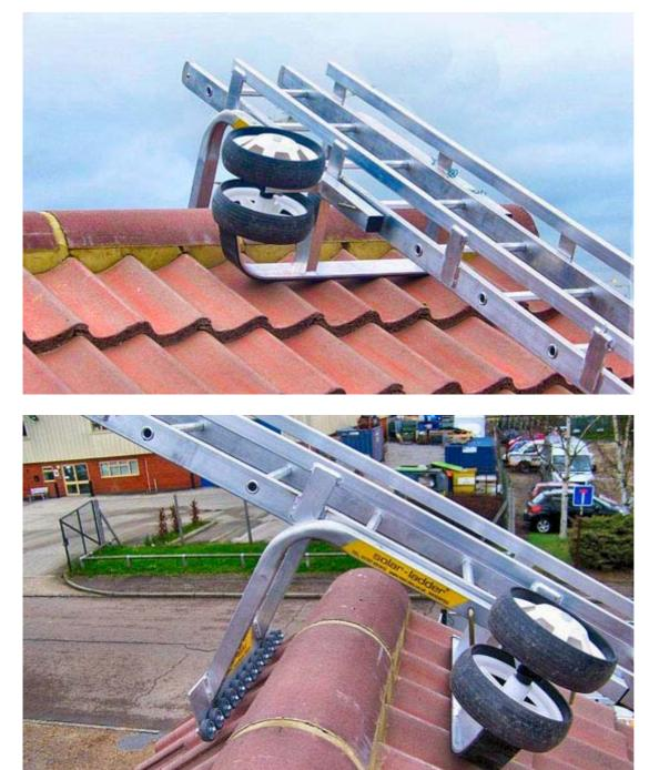
To use, simply roll ladder up the roof on it's soft rubber wheels and then flip 90° into position over the ridge. The special roof hook can be fixed to any rung, enabling the ladder to fit any size roof with the excess length flying out beyond the ridge.
