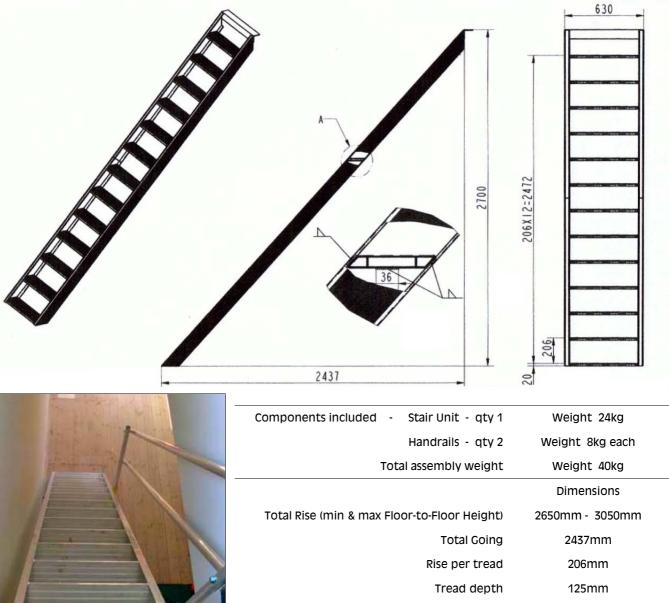
Width excl handrails 630mm Overall width incl handrails 730mm
