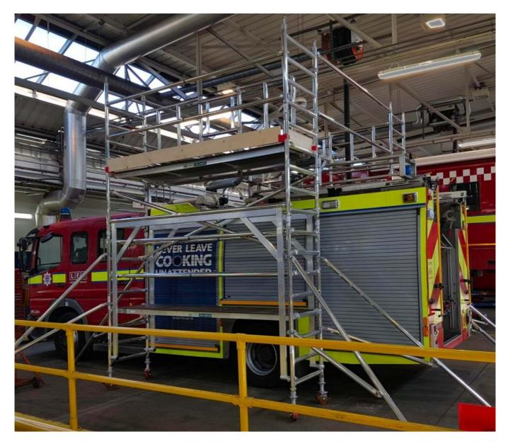
Twin Single Width Alloy Scaffold Towers fitted with high clearance base frames and narrow cantilever frames on their inner face are then linked with long guardrails to create a safe, guardrailed environment for maintenance work on larger vehicle roofs.
