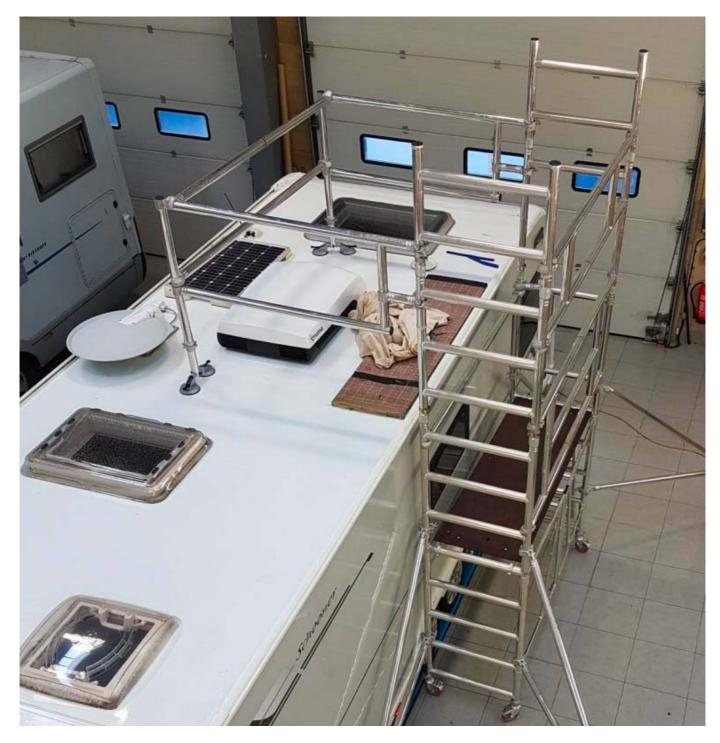
Single Width Alloy Scaffold Towers combined with bespoke frames onto roof provides a safe, guardrailed environment for maintenance work on many types of vehicle roof.
